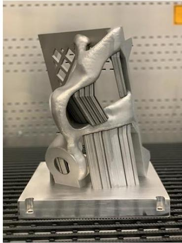
**Figure 9:** Mount for generative design bracket, with support material before post-processing.
