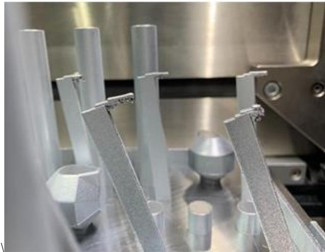
**Figure 1:** Example of high aspect ratio parts being pushed over due to a rigid re-coater blade.
