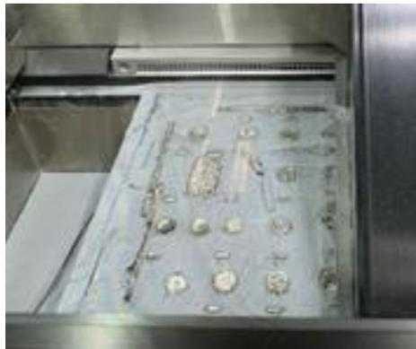
**Figure 4:** The results of the laser running over the parts when a new layer of powder has not been deposited.
