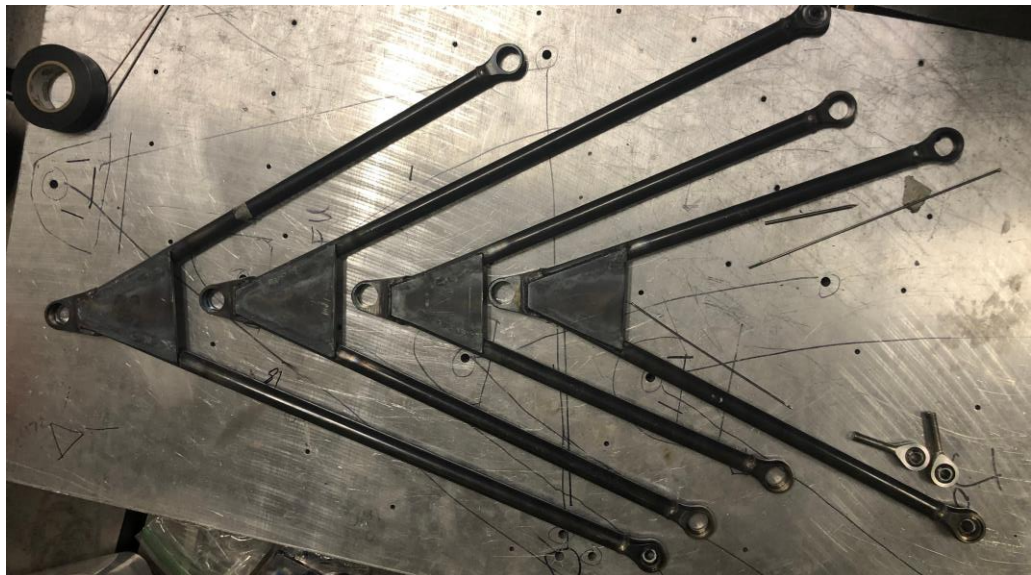
Figure 36: Lower Control Arms Welded and Assembled
