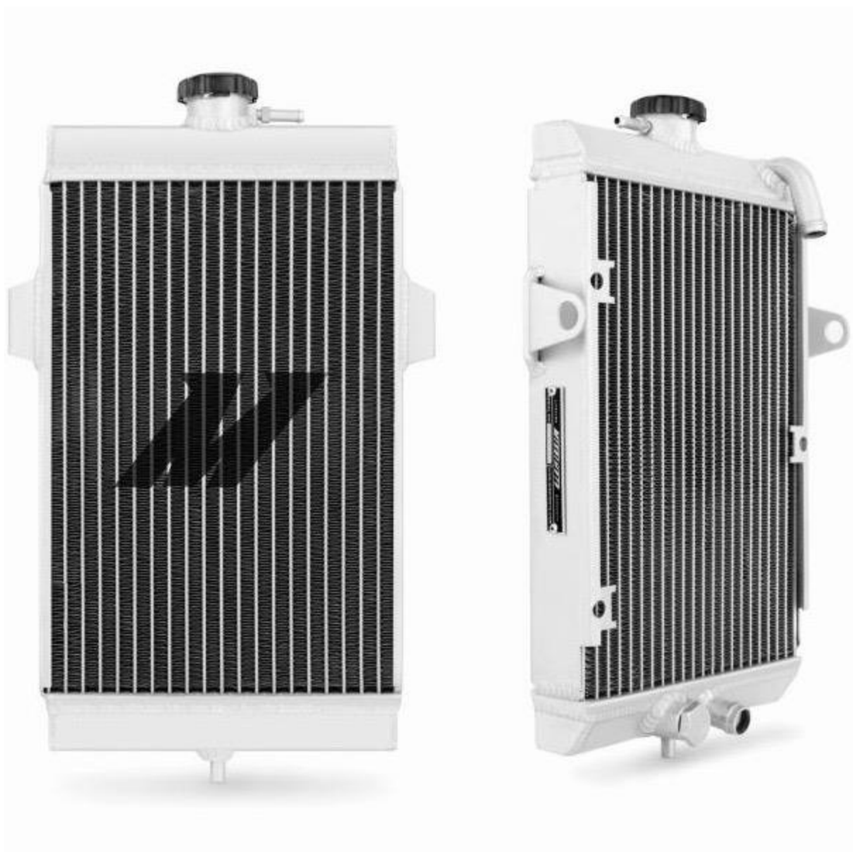
Figure 65: Mishimoto radiator selected for use on the 2019-2020 FASE car. (Mishimoto.com)
