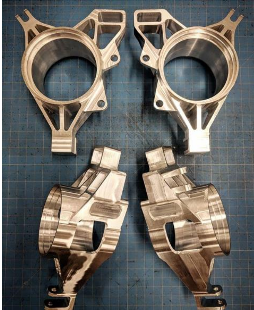
Figure 23: Completed Machined Uprights
