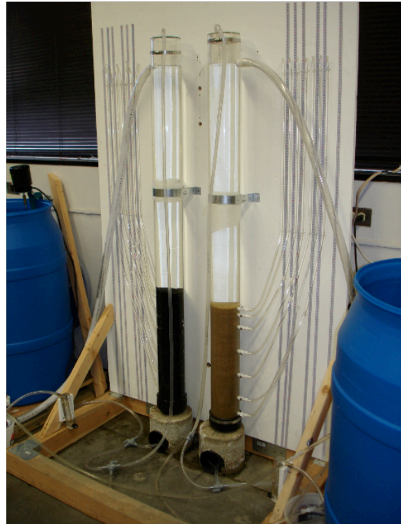
Figure 1: Parallel filter apparatus, showing tire crumb rubber media on the left, and filter sand on the right.
