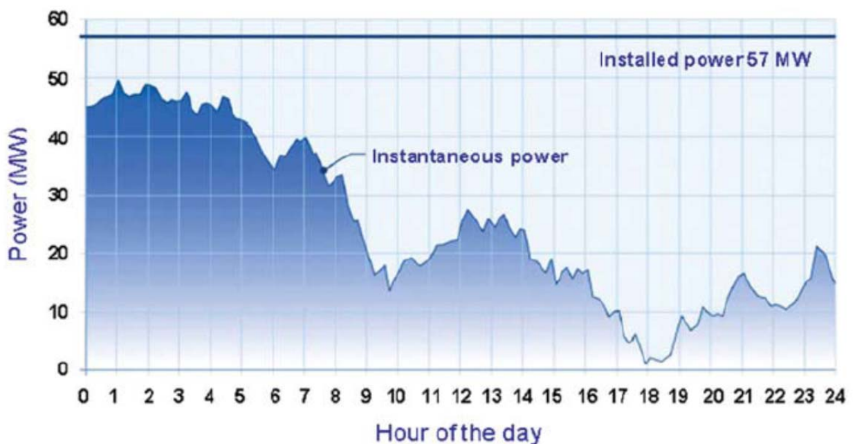
Figure 2. Instantaneous Power for a Sample Wind Farm in Canada – 76 Turbines (Ibrahim et al, 2007)
