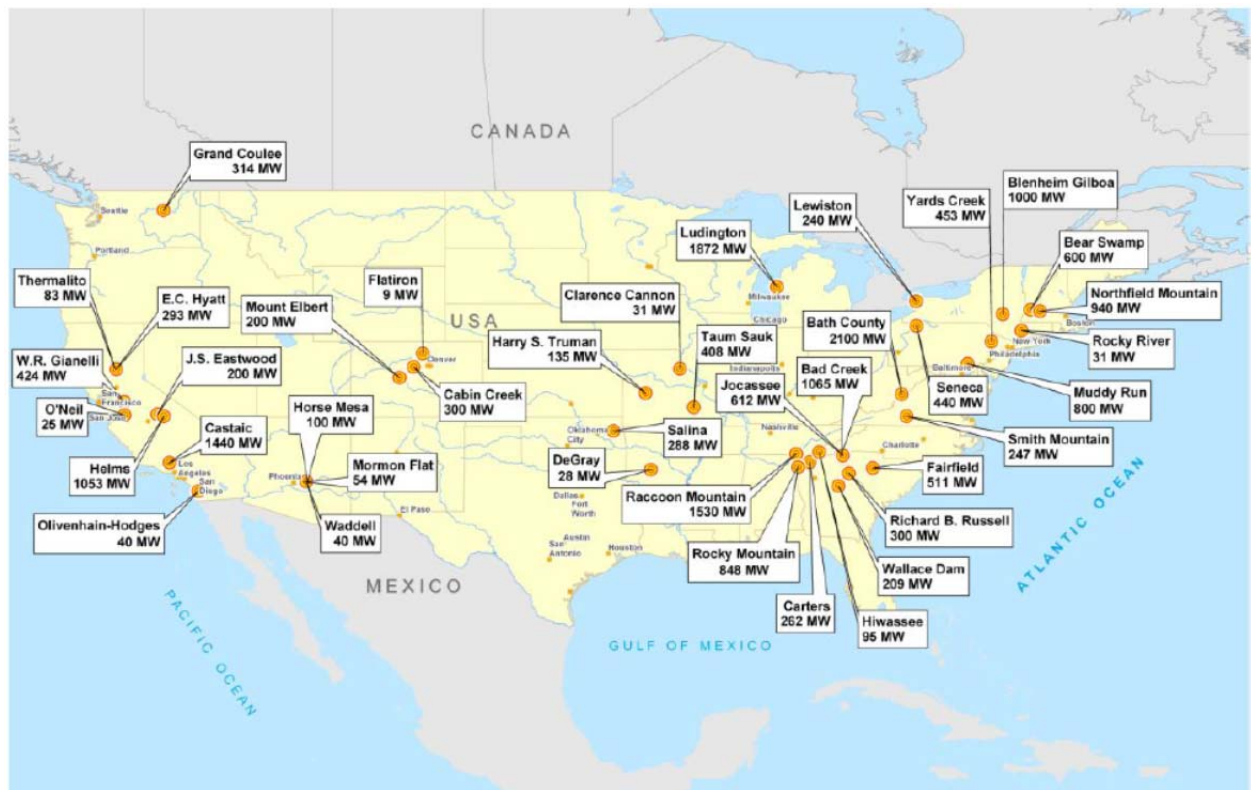
Figure 5. Existing Pumped Storage Hydropower Projects in the United States (Miller and Winters, 2009)
